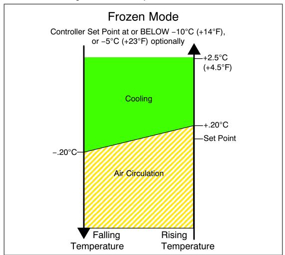
Figure 4.8 Controller Operation - Frozen Mode
