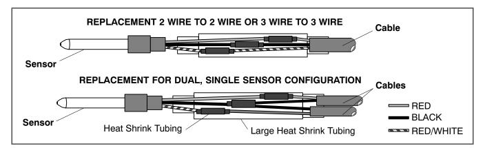
Figure 7.26 Sensor and Cable Splice
