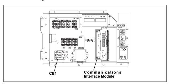
Figure 7.29 Communications Interface Installation
