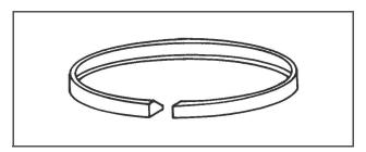
The gap between the ends of the piston rings can be checked with a feeler gauge by inserting the ring into the piston bore approximately one inch below the top of the bore. Square the ring in the bore by pushing it slightly with a piston. The maximum and minimum allowable ring gaps are 0.33 and 0.127mm (0.013 and 0.005 inch) respectively.
