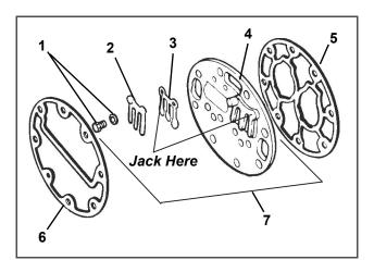
Figure 7.6 Exploded View of Valve Plate
