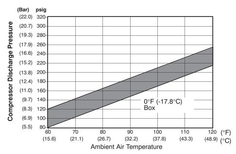
Compressor Discharge Pressure Versus Ambient Air Temperature at Stable Box Temperature
