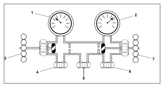
Figure 7.1 Manifold Gauge Set
