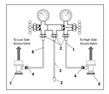
Figure 7.2 R-134a Manifold Gauge/Hose Set
