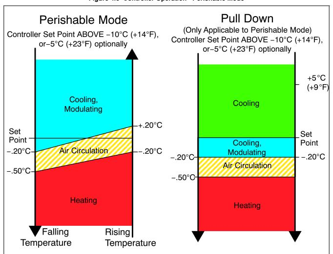
Figure 4.5 Controller Operation - Perishable Mode
