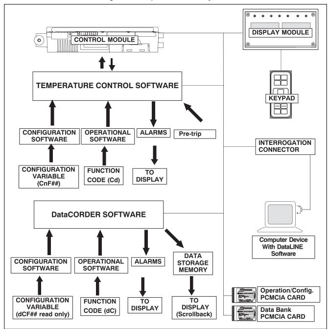
Figure 4.1 Temperature Control System
