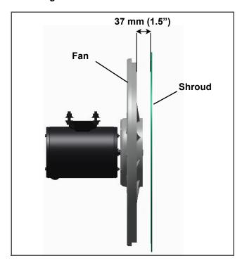
Figure 7.16 Condenser Fan Position
